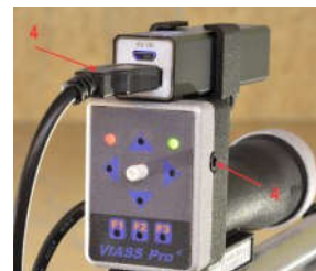
Step 4: Connect headphones and battery
